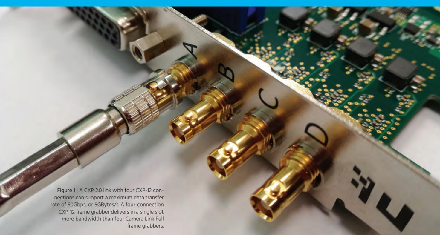
Figure 1 | A CXP 2.0 link with four CXP-12 connections can support a maximum data transfer rate of 50Gbps, or 5GBytes/s. A four-connection CXP-12 frame grabber delivers in a single slot more bandwidth than four Camera Link Full frame grabbers.
