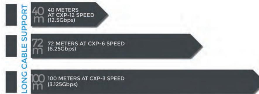
Figure 2 | Due to the efforts expended on cable drivers and equalizer to make CXP-10 and CXP-12 possible, the cable lengths for lower bitrates were significantly improved.
