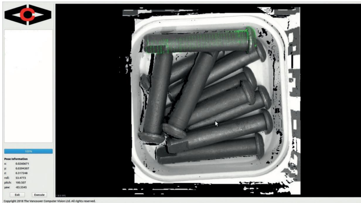
Image 1 | VCV-Cortex Pose estimation viewer. Showing a bin full of dark shiny rivets. The found rivet is highlighted in green and its 6D pose shown on the bottom left corner. Being a pre-trained AI system, it needs less than one minute to learn the geometry of any new part.
