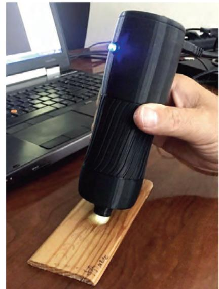
Figures | Micro Code uses a chemical labeling method in combination with optical authentication. The technology utilizes special markings detected by a product called Sova-UV1 (right figure). Image of a micro code in the software viewer (left figure).
